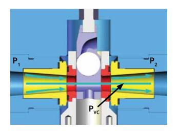
The illustration shows the typical change in pressure as the fluid moves through the valve. At inlet, the pressure is P<sub>1</sub>. Velocity increases through the valve to a maximum as it moves through the valve port. At the valve port, the pressure drops to  $P_{VC}$  (pressure at the vena contracta), which is the lowest pressure in the valve. As the fluid exits the valve, pressure recovers to  $P_2$  which is lower than  $P_1$ .
